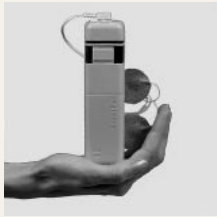
Figure 2. A capacitively coupled stimulation device. (EBI, Parsippany, NJ)
